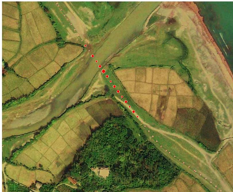
Satellite photo of a pipeline in river valley with severely damaged coating
